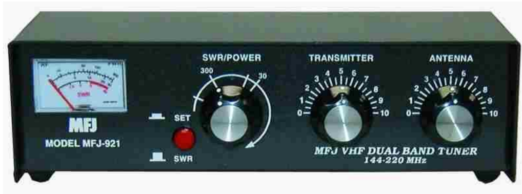
Antenna tuner VHFL πχ. 144-220 MHz
