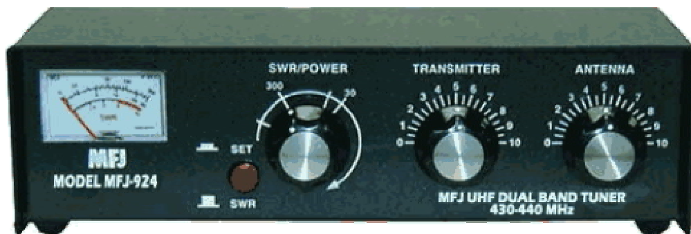
Antenna tuner UHF πχ. 430-440 MHz
