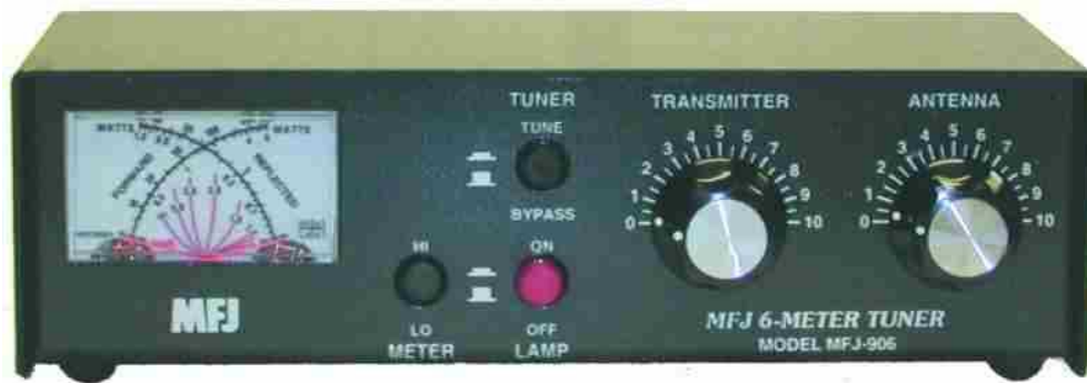
Antenna tuner VHFL πχ. 50 - 54 MHz
